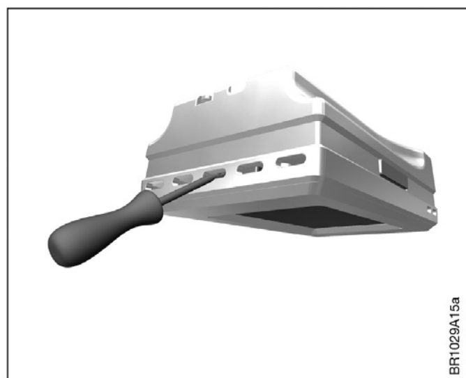
Fig. 2 Removing the front cover
